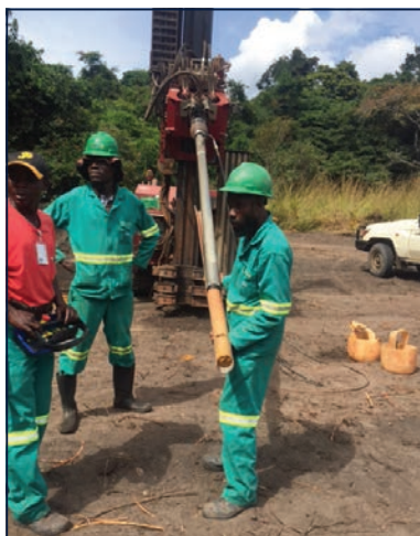
FIGURE 4. Full core recovery: sonic drilled in alluvial diamond prospects (northeast Angola).
