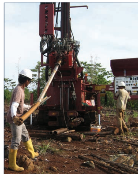
FIGURE 6. Sonic drilled core from Ni laterites (Weda Bay, Indonesia, ERAMET Group).
