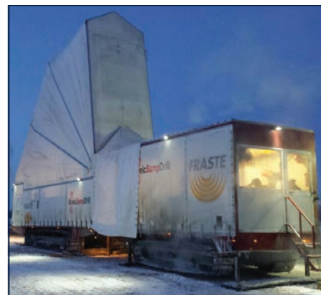
FIGURE 2. The LargeRotoSonic drill rig in the permafrost region of Far East Siberia hosting alluvial Au deposits.
