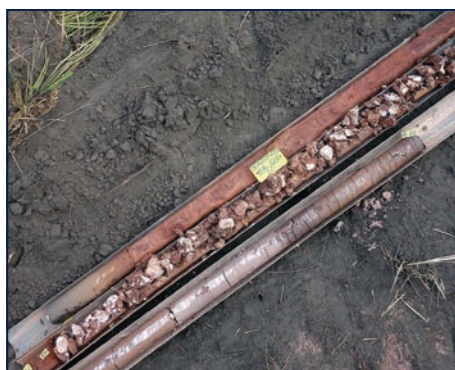
FIGURE 5. Full core recovery showing the gravel bed and country rocks (sonic drilled in alluvial diamond prospects, northeast Angola).
