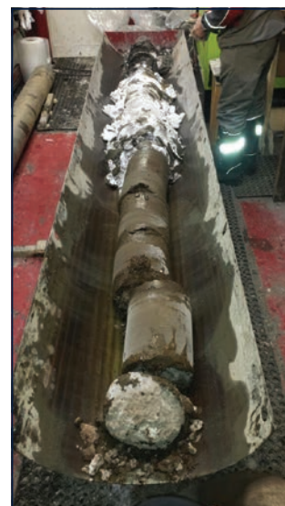
FIGURE 3. Sonic drilled cores in the permafrost region hosting alluvial Au deposits (Far East Siberia; Eijkelpamp SonicSampDrill).
