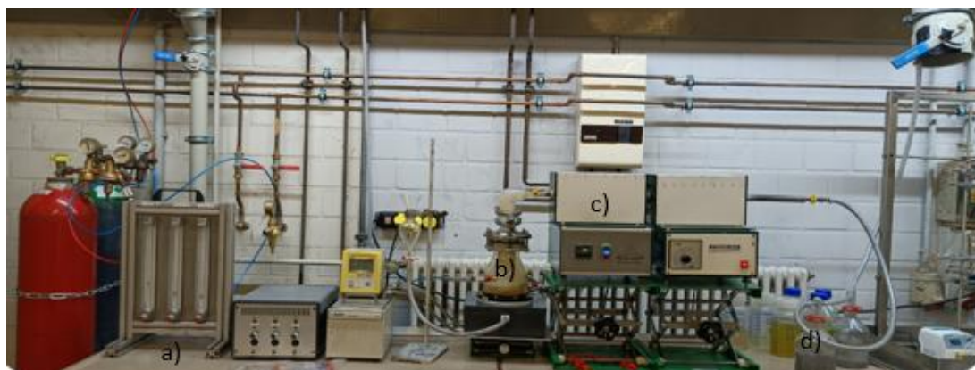
Figure 4. Scheme of USP equipment a) Gas flow regulation; (b) ultrasonic aerosol generator; (c) furnace with the wall-heated reactor; (d) collection bottles.
