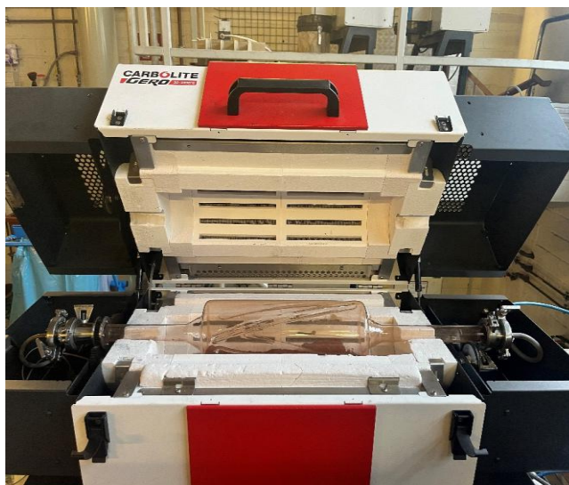
Figure 2. Rotary kiln for hydrogen reduction
