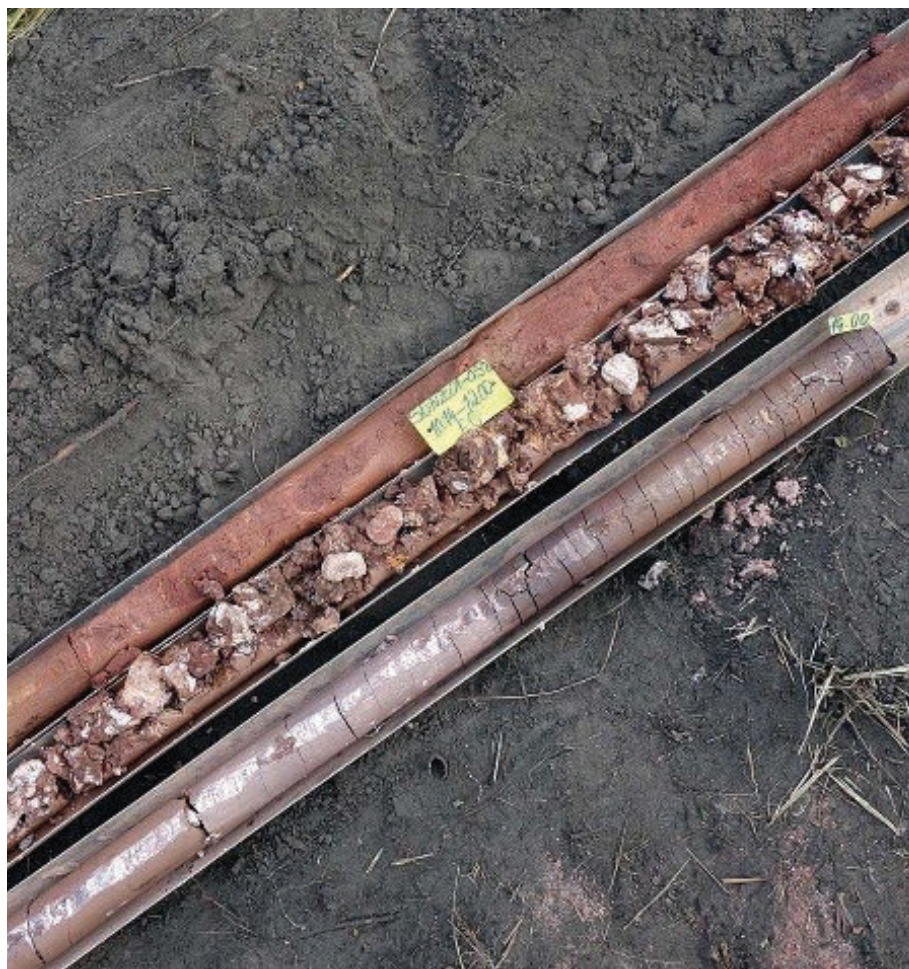
The samples made with Eijkelpkamp's sonic drilling technique
