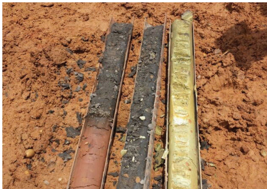
The samples made with Eijkelpkamp's sonic drilling technique
